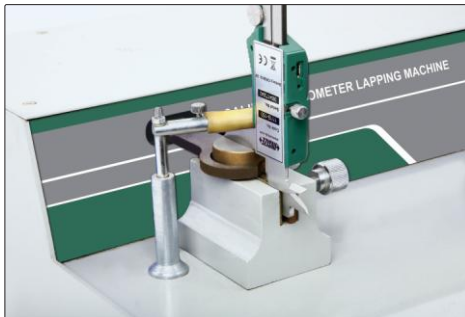
lapping measuring surfaces of caliper lower jaws
