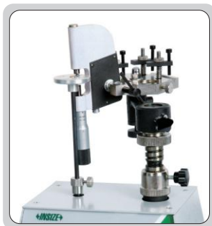
check the measuring force of indicating micrometers
