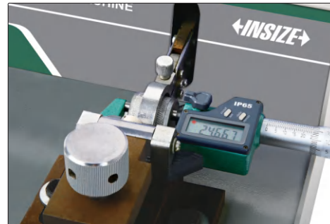
lapping measuring surfaces of outside micrometer
