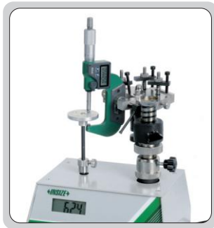
check the measuring force of micrometers
